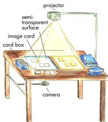
Figure 1. Setup of the Tangible Interface.
