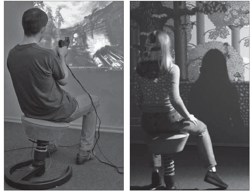
Figure 1. The ChairIO used as gaming input device. Here, the Swopper™ from aeris-Impulsmöbel GmbH is used as the basis for the ChairIO. User playing a First-Person-Shooter with the ChairIO and gun interface (left). User playing a Jump'n'Run Game (right).
