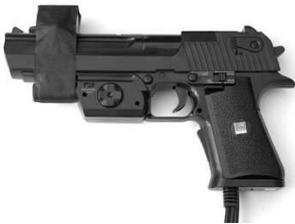
**Figure 2. Gun Interface with d-Pad, Buttons, Trigger, and Orientation Tracker.**
