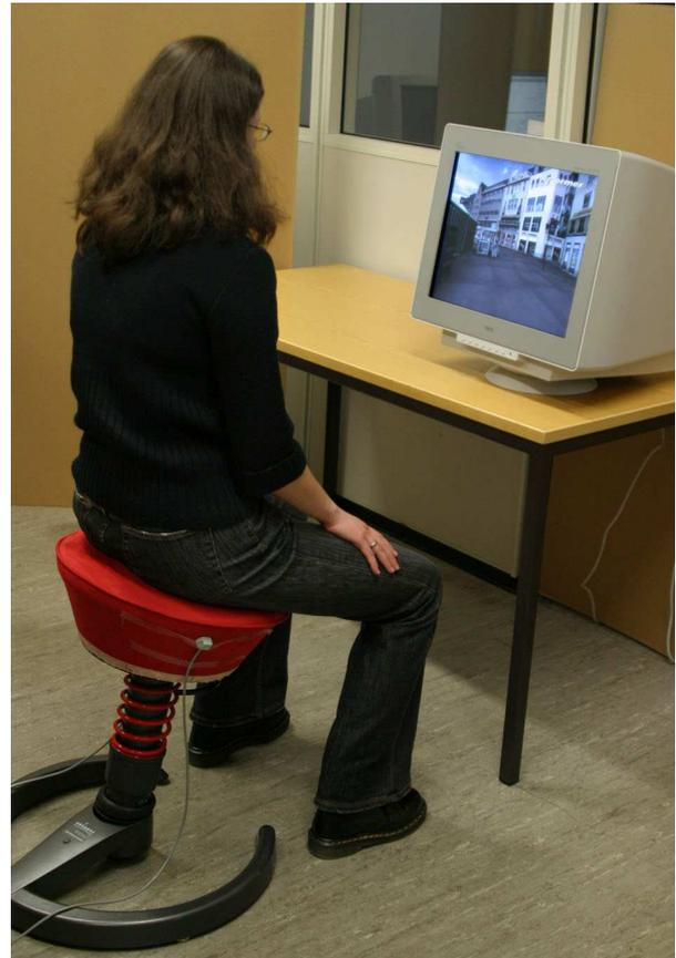
**Figure 3. Chair Interface Used for Travel in VE.**
