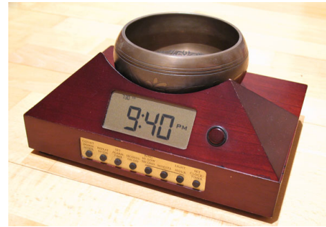
Figure 3. Zen Timepiece is a digital alarm clock that slowly wakes people with a real brass bowl-gong. The time intervals between gongs decrease in a harmonious function.
